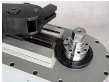
Permutable shaft The PT series is equipped with permutable shaft for tight radius.
