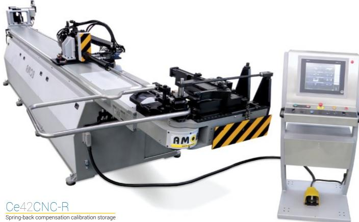
CNC hydraulic pressure die assist Programmable variable radius
